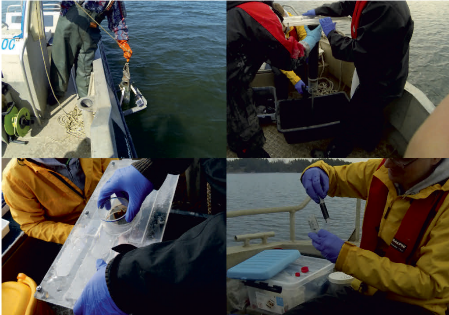
Photo 2 The sampling campaigns generally included sampling of sediment cores and collecting the cores for incubation back in the laboratory (upper left and right). Additionally, some cores were sacrificed in the field by slicing various sediment depths (lower left) and collecting the sediment in different tubes for further chemistry and molecular determinations (lower right). Photos are used with permission and were taken by the Linnaeus University Coastal Group.
