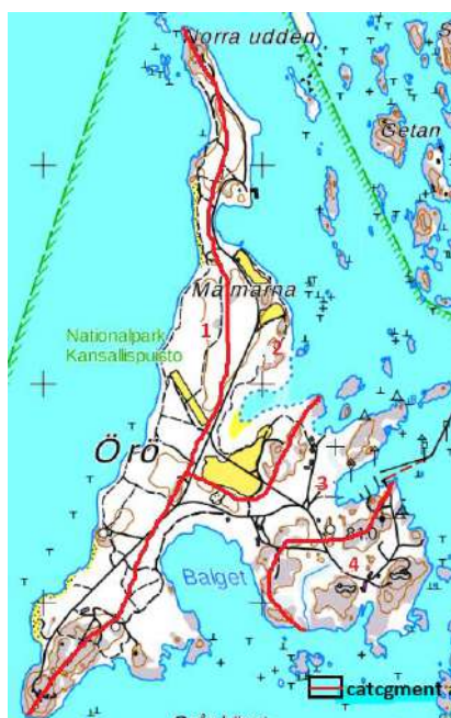
Figure 5. The main catchment areas (1-4) in Örö where the groundwater recharge can be found.
